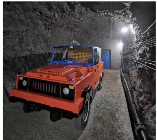
*Figure 1: Rubber-tired general-purpose vehicle for underground transportation*
